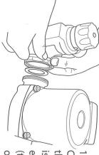
ensuring the pump washer is inserted is pre-assembled to the thermomix, on the pump body) (taking note of the directional arrows the pump using the pump nut which Connect the Thermomix UFH valve to
